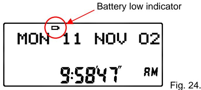
\*\* : Only replace the CR2032 with the 4 pieces AA Batteries installed or with the AC adaptor plugged. This can retain the timer's memories and settings.
